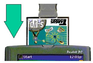
The card should fit easily into the CompactFlash card slot. If you encounter resistance, make sure the card is aligned correctly (top facing you).
