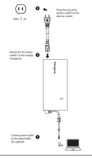
NOTE: YOUR TARGUS LAPTOP CHARGER (A) WILL AUTOMATICALLY ADJUST **THE WATTAGE TO MEET** THE SPECIFICATIONS OF YOUR LAPTOP (UP TO 90 WATTS) AND BEGIN CHARGING YOUR LAPTOP BATTERY, YOURLAPTOP **CANBEPOWEREDONAND** IN USE WHILE THE ADAPTER CHARGESTHE BATTERY. AFTER UNPLUGGING YOUR ADAPTER, PLEASE WAIT AT LEAST5SECONDS BEFORE PLUGGING IT BACK IN TO ALLOWITTO RESET.
